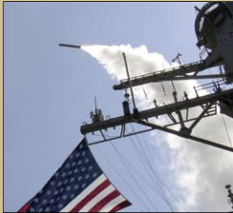
Figure 1 A Tomahawk Land Attack Missile (TLAM) is shown here launched from the U.S. Navy Arleigh Burke Class Guided Missile Destroyer, USS Porter (DDG 78). (DoD photo).
