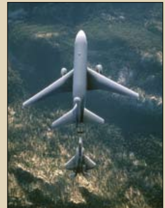
Figure 2 A KC-10 Extender aircraft, from Travis Air Force Base, CA, refuels an F/A-22 Raptor. (U.S. Air Force photo).
